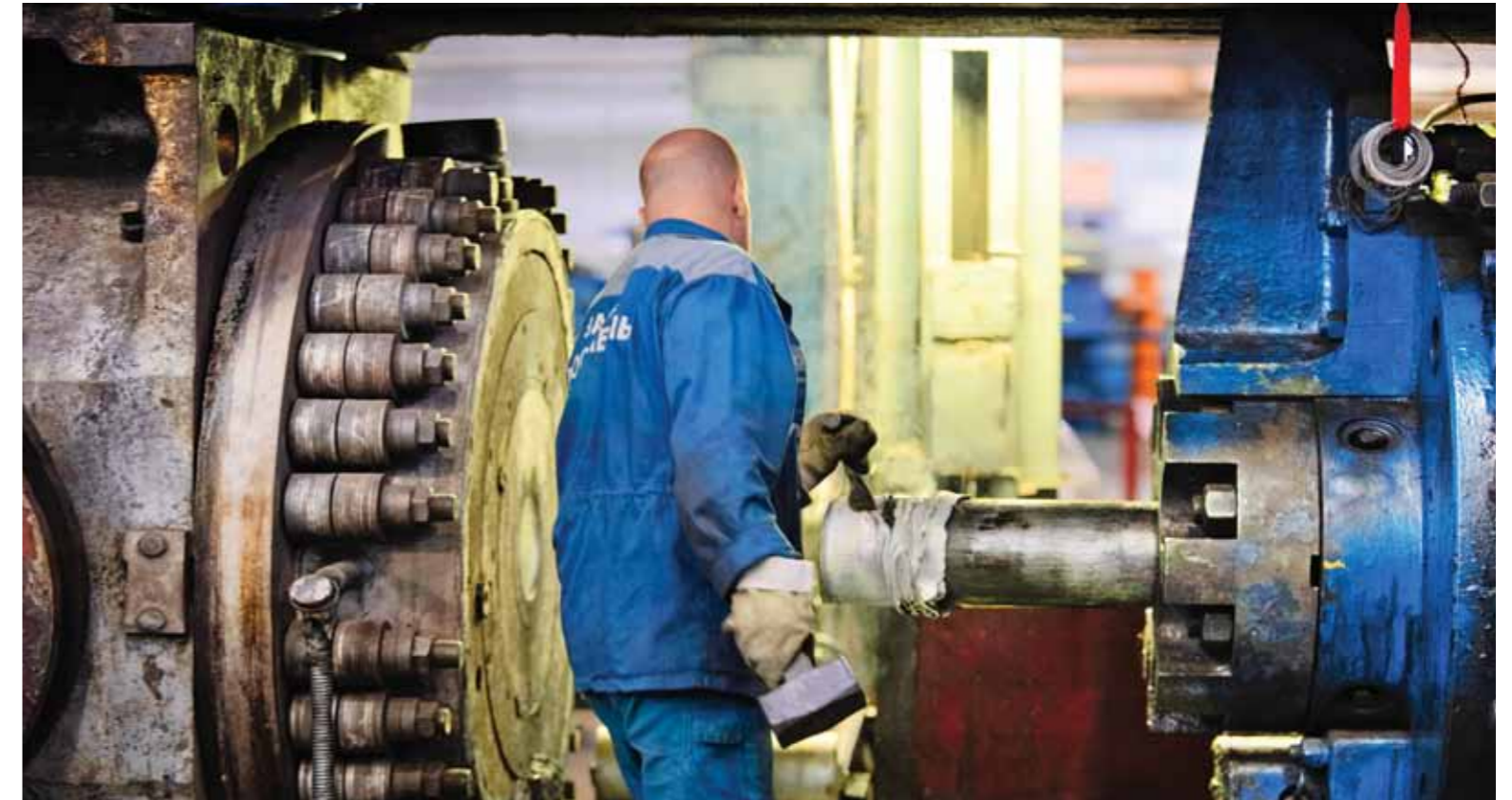
Operation of Pressing Aluminium Power Cores
