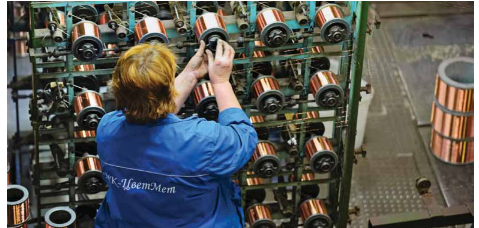
Installation of Payoff Reels with Wire in the Process of Manufacturing Wires for Brushes of Electrical Machines of PShch Brand
