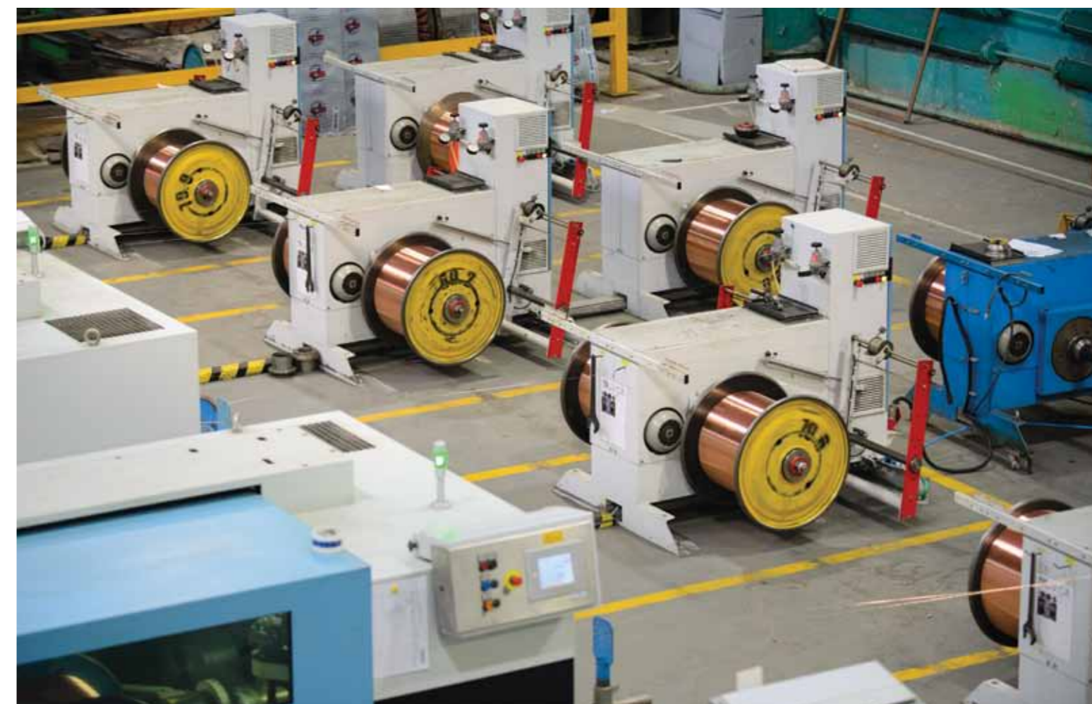
Modern Line of Multi-Circular Drawing and Twisting for the Production of Copper Conductors
