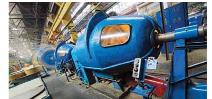
The Process of Applying Protective Coatings on Cables with Paper Impregnated Insulation
