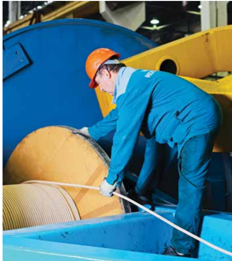
Operation of General Twisting of Cables with Polymer Insulation
